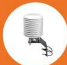
Ambient Temperature & Humidity with Solar Shield
